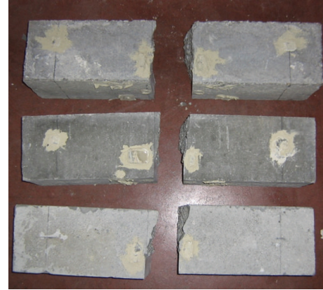
FIGURE 6: Post-test aspect of the notched specimens without fibres.
