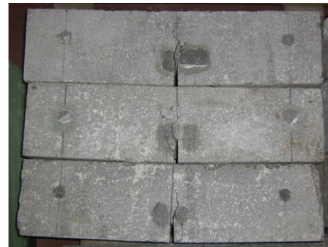
FIGURE 7: Post-test aspect of the notched specimens with 1% of steel fibres volume content.
