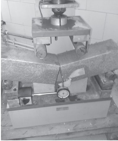
FIGURE 3: Brittle break of specimens without a fiber core (PC2).
