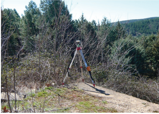
FIGURE 3: GPS receiver at the reference base near the construction.
