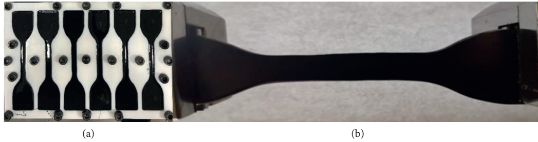
FIGURE 2: Dumbbell shape (a) and tensile details (b) of the test samples.
