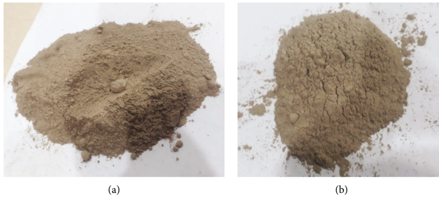
FIGURE 3: Powdered ladle furnace slag (LFS) used in this study (a) raw LFS powder; (b) sieved (#200) LFS powder.
