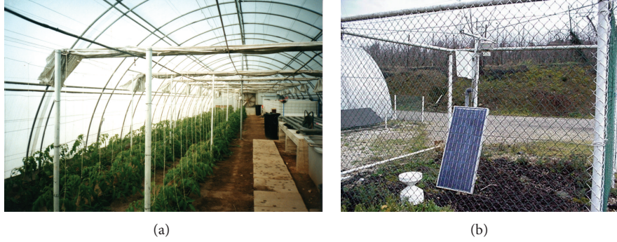
FIGURE 1: The experimental setup: a greenhouse with floor area of 210 \text{ m}^2 (a). Indoor temperature, relative humidity, soil temperature, and \text{CO}_2 are measured. In the outside, wind speed, outside air temperature, relative humidity, and solar radiation are measured by a weather station located in the greenhouse vicinity (b).
