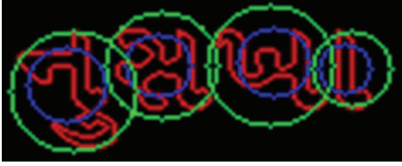
FIGURE 6: Computation of circularity of component on Gujarati script using fitted circles (blue: minimum encapsulating and green: best fitted).
