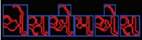
FIGURE 7: Computation of rectangularity of component on Gujarati script showing blue: rectangular box.
