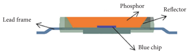
FIGURE 3: Schematic representation of the package with phosphors and a blue LED chip used in the simulation.
