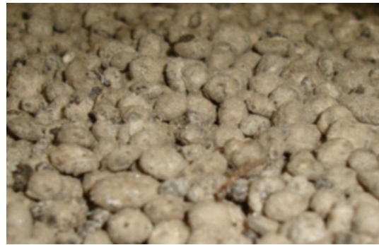
FIGURE 2: A sample of OMF 15 with particles in the range of 1.18 to 5.50 mm in diameter.
