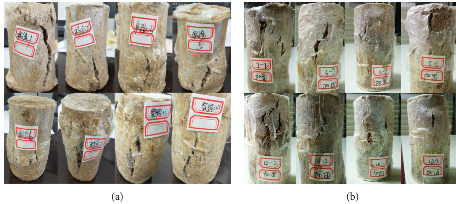
FIGURE 8: Splitting failure of specimens under uniaxial compression. (a) CCS and (b) CFS.
