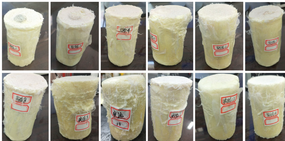
FIGURE 7: Plastic failure and deformation of PCS.
