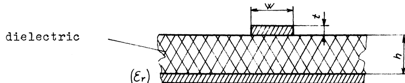
FIGURE 6 Asymmetrical microstrip transmission line. \epsilon_r = relative dielectric coefficient.
