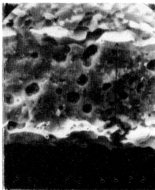
FIGURE 14 Cross-section showing high porosity of dielectric DP 19120-123. Magn: x1200, Secondary electron image (25 kV).
