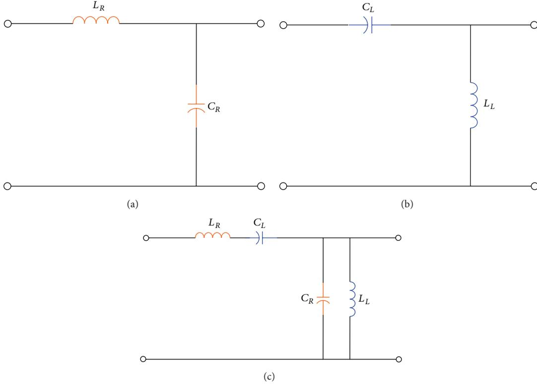
FIGURE 1: Equivalent circuits: (a) pure RH TL, (b) pure LH TL, and (c) CRLH TL.
