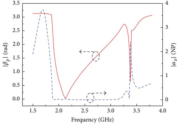
FIGURE 6: Dispersion characteristic diagram of the designed filter with improved CRLH structure.
