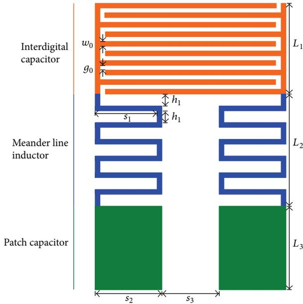
FIGURE 3: Microstrip implementation of the improved CRLH structure.
