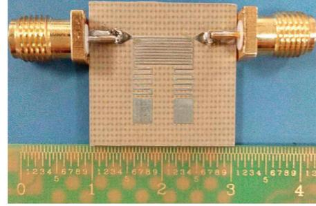
FIGURE 4: Photograph of the proposed filter.
