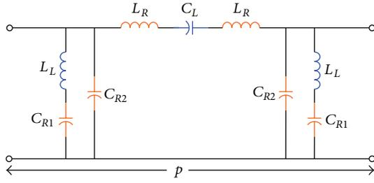
FIGURE 2: Symmetrical equivalent circuit of the improved CRLH structure.
