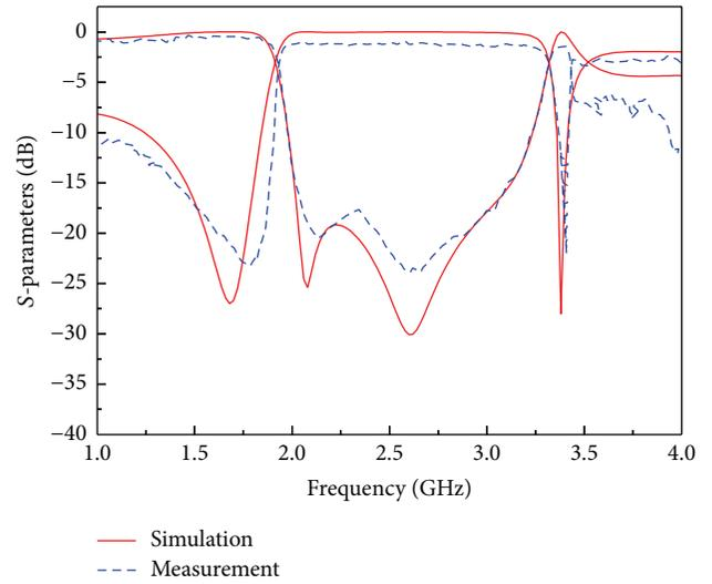
FIGURE 5: Measured and simulated responses of the wide-band filter.
