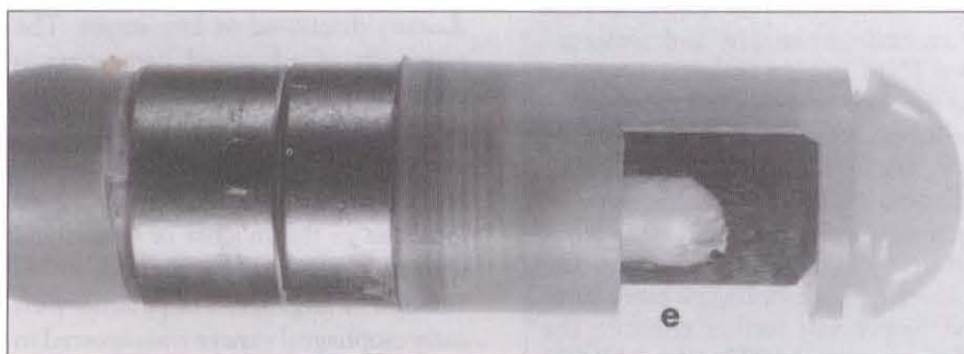
Figure 2 A flexible nonoptic Aloka ultrasonic instrument with a small echoprobe (e) at the tip
