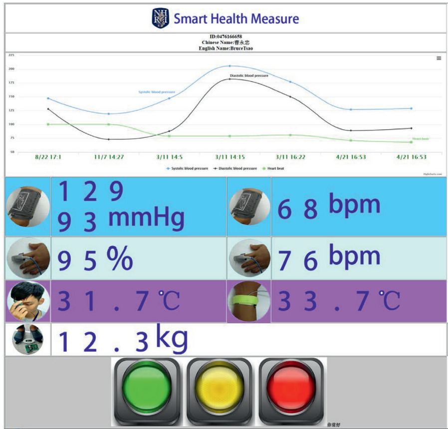
FIGURE 5: User profiles and physiological health parameters (essential vital signs) kept in the cloud platform developed in this paper. First, users access the website through a browser with their health ID card. The website generates visualized reports based on the measured data and displays a chart of data collected over the previous seven days to visualize the blood pressure trend. Other data can also be displayed side by side. User health is indicated by a red/yellow/green light indicator similar to a traffic signal for analysis and is then summarized from the user profiles and physiological health parameters. Users can also click on icons under the chart in Figure 5 to view the detailed data as a separate chart.
