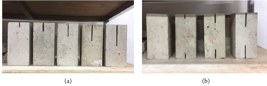
FIGURE 1: Rock-like specimens with different cracks: (a) specimens with unilateral crack; (b) specimen without crack and specimens with bilateral crack.
