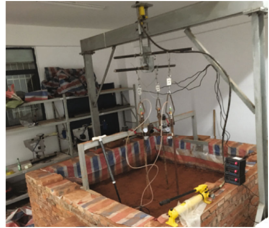
(b) Three-anchor test ( G_{three} )
