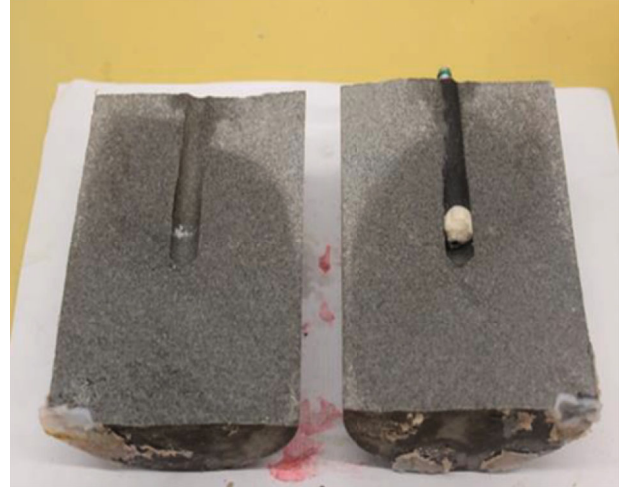
FIGURE 6: The vertical fracture created along the axial direction in a specimen for the first batch.
