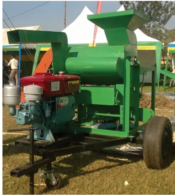
FIGURE 5: SIL’s multicrop thresher that processes maize and soybean as well as other crops [109].
