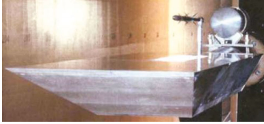
FIGURE 1: Noise test of M219 cavity in wind tunnel.
