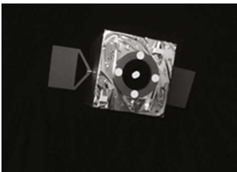
FIGURE 13: An image of the satellite model captured by the monocular camera.
