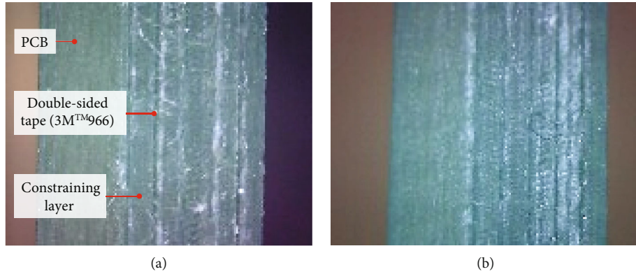
FIGURE 16: Representative optical microphotographs of the solar panel side edge: (a) before TV environment test and (b) after TV environment test.
