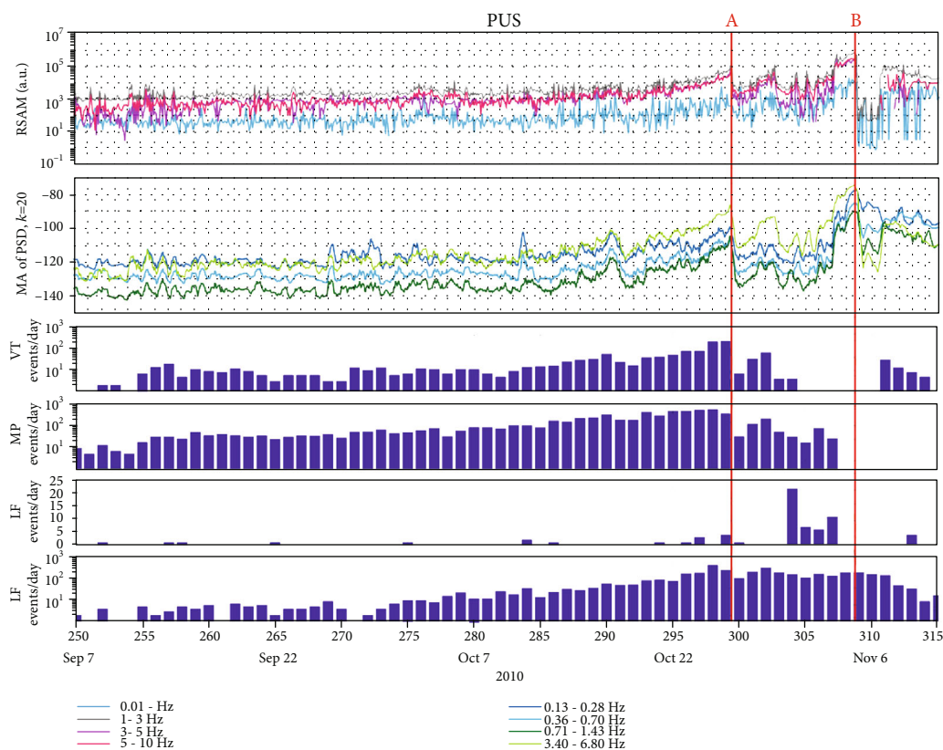
FIGURE 10: Comparison of analysis results using RSAM, temporal variation of PSD, and daily number of events calculations of volcano-tectonics (VT) A+B, multiphase (MP), low-frequency (LF), and rockfalls (RF) during the Merapi eruption period 2010. The RSAM result and the daily event observation were carried out by BPPTKG [2]. It can be seen that the PSD calculation is able to show fluctuations in volcanic activity mainly related to the amount of VT, MP, and RF events better compared to RSAM calculation.
