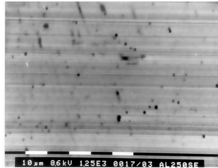
Figure 3. Defects observed in 750 °C annealed samples.
