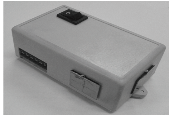
FIGURE 10: The proposed sun-tracking sensor.
