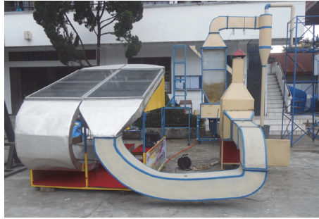
FIGURE 1: Photograph of the solar assisted heat pump fluidized bed dryer integrated biomass furnace.
