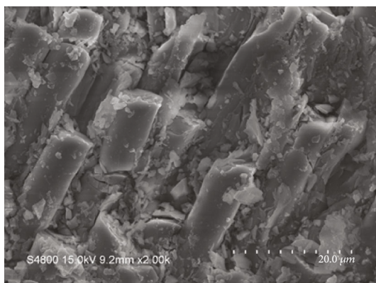
FIGURE 3: SEM of fractured surfaces of MDPES-2 composite ( \times 2000 ).
