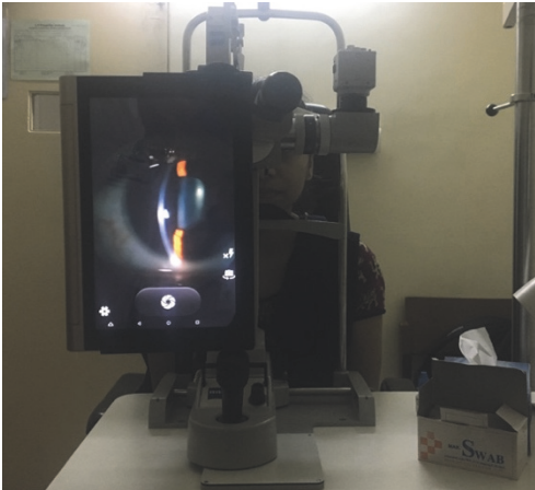
FIGURE 15: eyeSmart Cyclops attached to the slit lamp.
