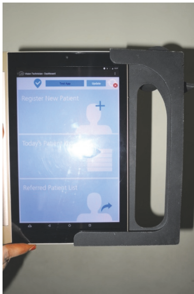
FIGURE 11: Insertion of tablet into eyeSmart Cyclops.
