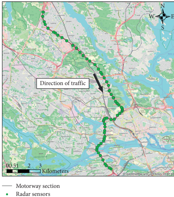
FIGURE 2: Modelled motorway section and the sensors' position.
