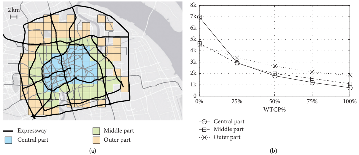
FIGURE 10: Truck flow of different parts of Shanghai. (a) Study area divided into three parts and (b) truck flow (in- and out-flow) of each part.
