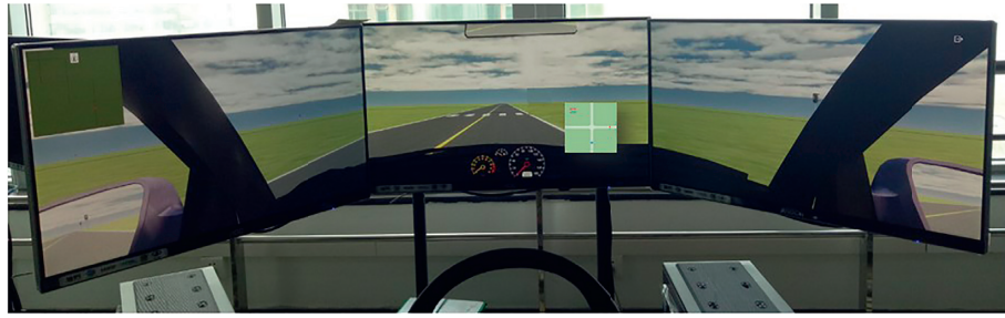
FIGURE 5: Display of the driving simulator and the warning interface.
