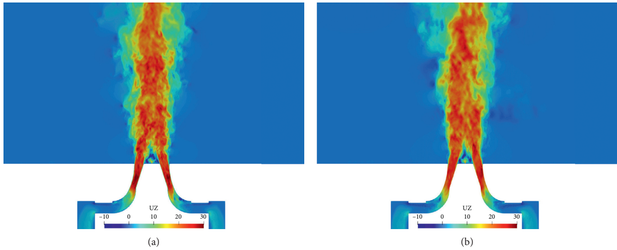
FIGURE 6: Instantaneous axial velocity fields for cases A-NR (a) and B-NR (b) in the central vertical plane.
