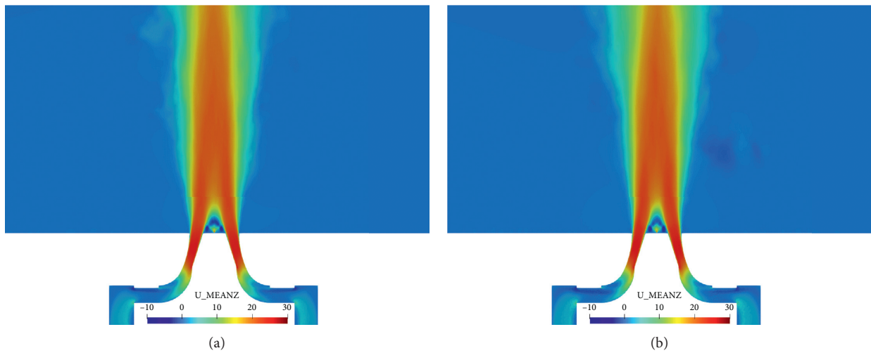
FIGURE 7: Mean axial velocity fields for cases A-NR (a) and B-NR (b) in the central vertical plane.
