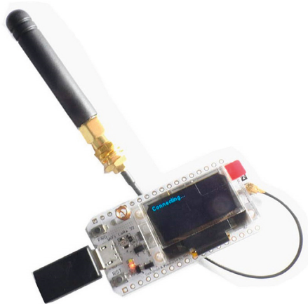
FIGURE 4: Selected microcontroller card, HiLetgo ESP32 LoRa 0.96 inch OLED display (Heltec).
