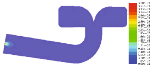
FIGURE 8: Contours of velocity distribution (m/s).
