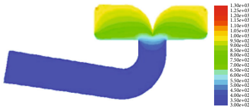
FIGURE 6: Contours of static temperature along the burner.
