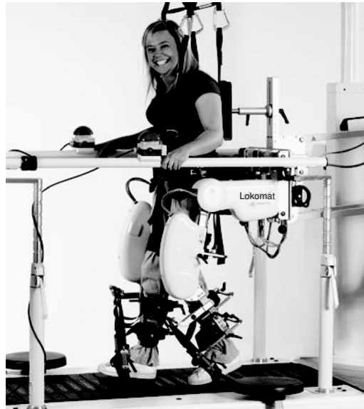
Figure 1b. Current version of the Lokomat system with spinal cord injured patient (2007).
