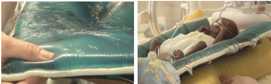
Figure 7. A mat of polyurethane gel with embedded sensors for the recording of interfacial pressures of specific anatomical points, temperature, and movements. The gel has anti-decubitus-ulcer properties because it distributes interfacial pressures in a larger surface area with respect to standard foams and with isotropic behavior so relieving the contact points on the body.
