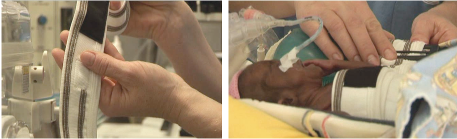
Figure 6. A wearable and sensitized band equipped with a set of sensors for monitoring newborn vital parameters including heart rate, breathing rate, temperature, and respiratory movements. The fabric is soft and extremely thin, and the sensors used are electrodes and extensometers, while the transducers are generic accelerometers and temperature sensors for medical use. The BioBelt permits a variety of measurements without having to paste, fasten, or position anything on the newborn but the belt itself.
