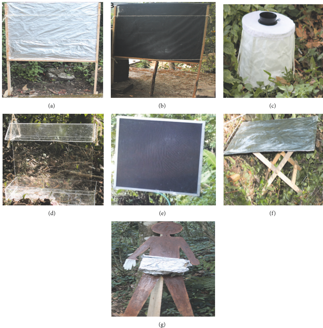
FIGURE 3: Traps evaluated by Rodriguez-Perez et al. (2013) for their potential in collecting S. ochraceum s.l. females in Mexico. (a) Vertical Bellac Plaque Trap. (b) Esperanza Window Trap (original). (c) BG Sentinel. (d) Clear Window Trap. (e) Esperanza Window Trap (acrylic/hanging version). (f) Horizontal Bellac plaque. (g) Human silhouette trap [source: Rodriguez-Perez et al., 2013].
