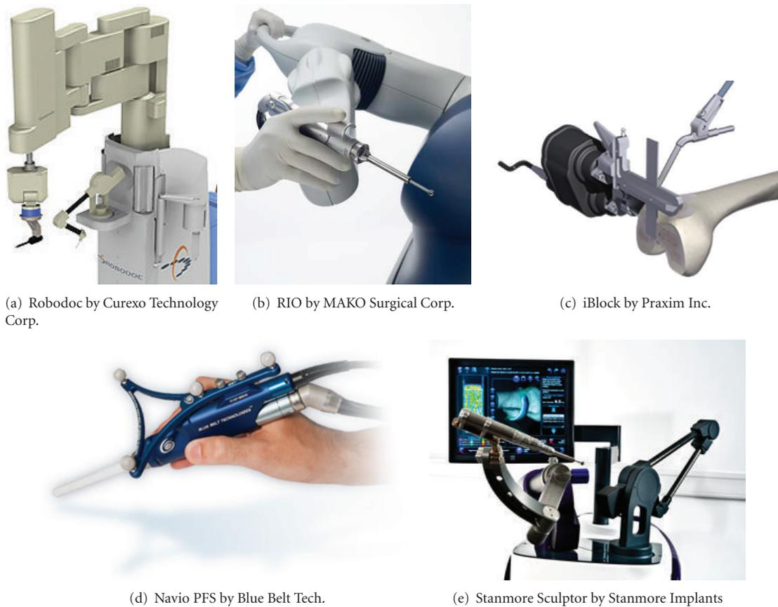
FIGURE 2: Orthopedic robots for accurate bone resection. The Robodoc image is ©2012 Curexo Technology Corp. The RIO image is ©2012 MAKO Surgical Corp. The iBlock image is ©2012 Praxim Inc. The Navio PFS image is ©2012 Blue Belt Tech. The Stanmore Sculptor image is ©2012 Stanmore Implants.
