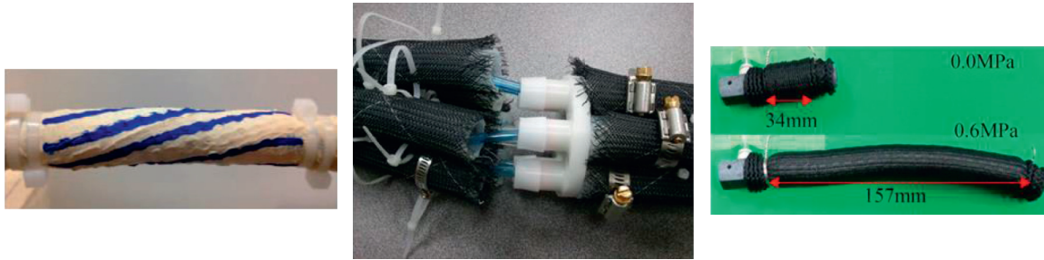
FIGURE 8: Pneumatic artificial muscle—fiber material and braided structure [206–209].
