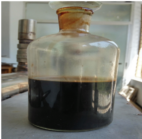
FIGURE 2: Crude tire pyrolysis oil from waste tire.
