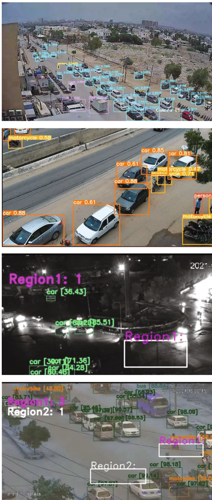
FIGURE 3: Detection results from the designed algorithms. Each object has a bounding box drawn over it, and a label is assigned by classification.
