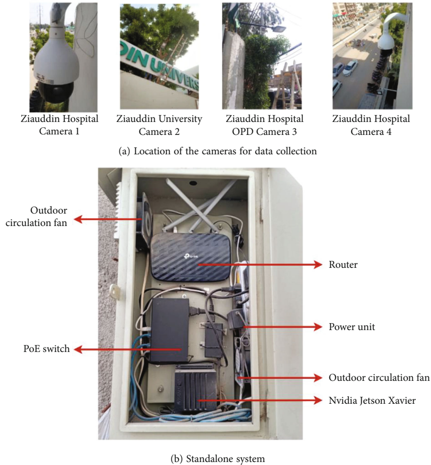
FIGURE 1: Locations of camera and hardware prototype of the proposed system. (a) Top picture shows the dataset collection performed from different Ziauddin university and hospital locations by placing the cameras. (b) Bottom image shows the processing unit being used in performing the proposed method.
