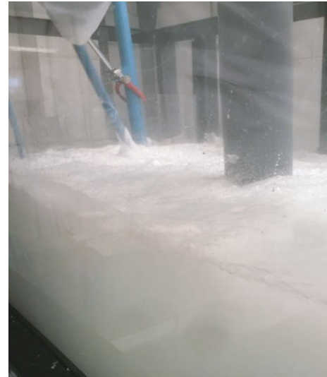
FIGURE 10: Microsphere flotation operation.
