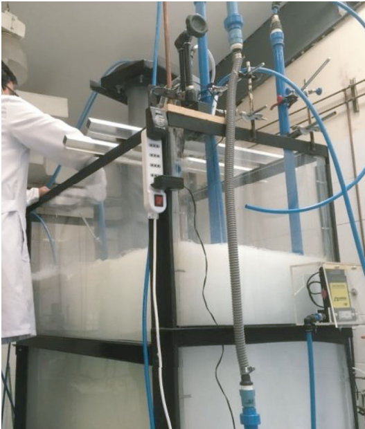
FIGURE 9: Flotation cell microsphere system.
