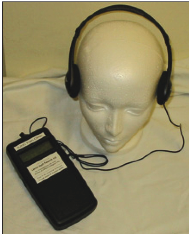
Figure 1) Headset for delivering pulsed electromagnetic fields or sham treatment
