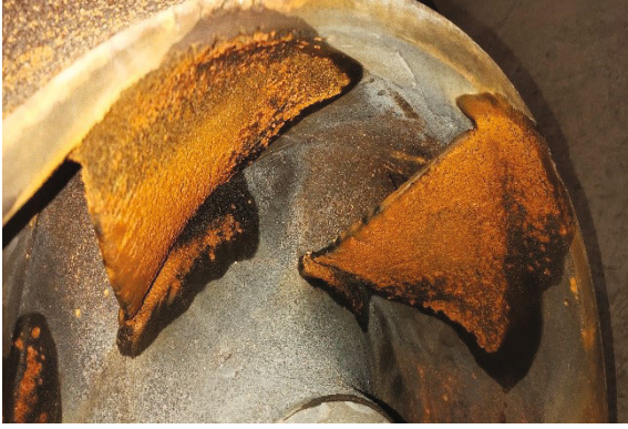
FIGURE 1: Cavitation erosion in the centrifugal pump.
