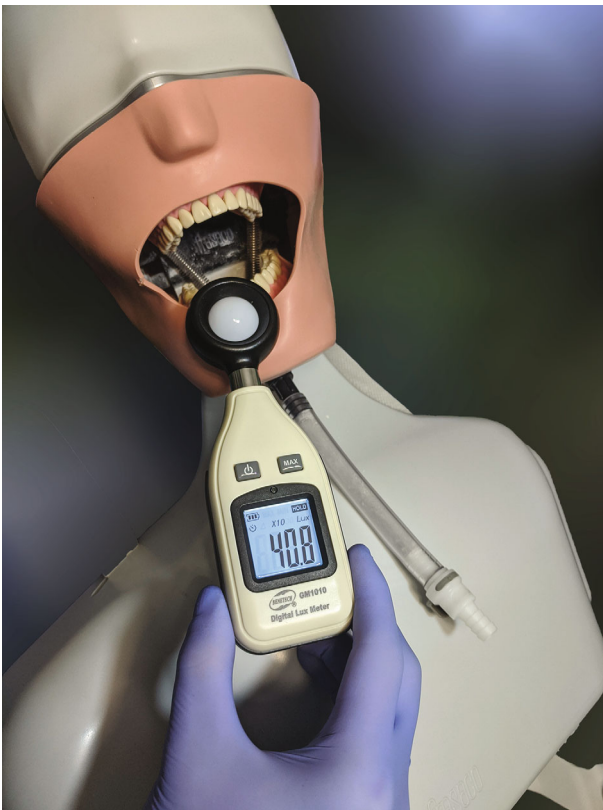
FIGURE 2: The lux meter GM1010 measuring the light intensity in the area of the typodont.
