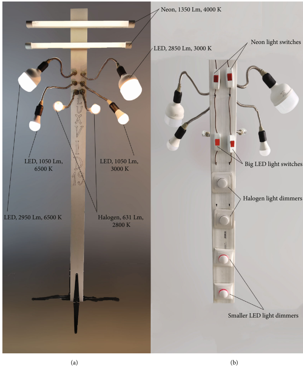
FIGURE 3: Lighting device named "Luxvid 19" designed specifically to aid in this study: (a) front view; (b) back panel containing the switches and dimmers.
