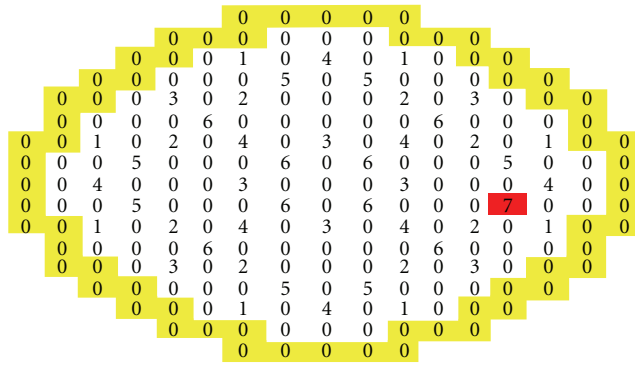
FIGURE 4: Control rod banks configuration.
