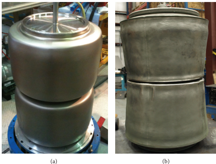
FIGURE 7: An ANSTO dumbbell design HIP can (100 L capacity) containing over 170 kg of Synroc waste form, before HIPing (a) and after HIPing (b), which was produced to demonstrate the scalability of HIPing.
