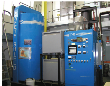
FIGURE 2: A hot Isostatic press located at ANSTO. This press can take up to a 30 cm diameter load. The machine consists of a pressure vessel in which a furnace is installed. Densification occurs under Ar at up to 200 MPa at the desired temperature.
