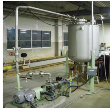
FIGURE 2: Photograph of the experiment centrifugal pump system.
