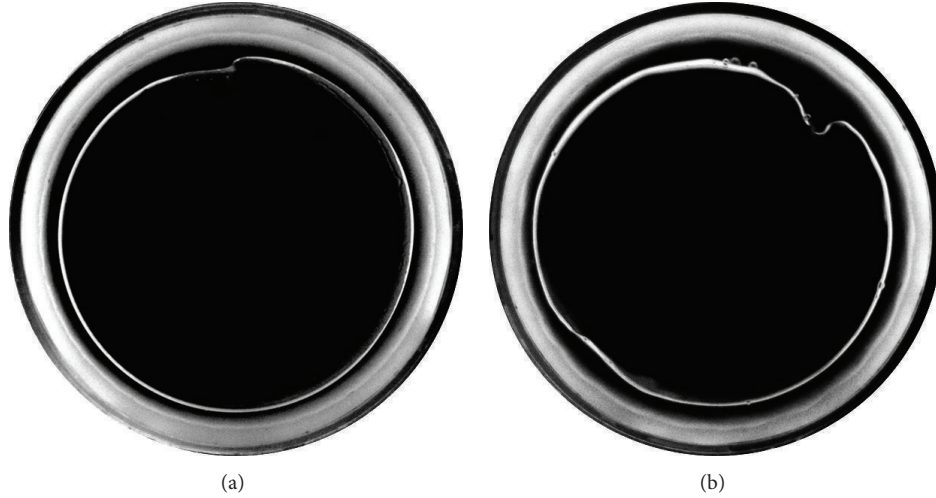
FIGURE 2: The azimuthal inertial waves (front view): l = 1 , q = 0.236 , and \Omega = 32.0 \text{ s}^{-1} (a) and l = 2 , q = 0.247 , and \Omega = 31.4 \text{ s}^{-1} (b); \nu = 3.2 \text{ cSt} and m = 250 \text{ g} , hereinafter cylinder rotates counterclockwise.
