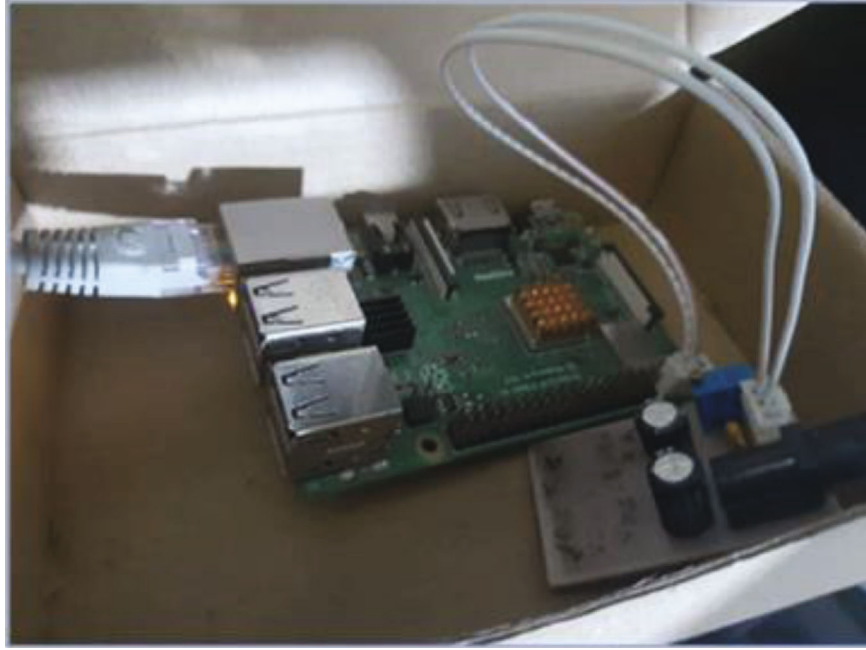
FIGURE 3: Raspberry Pi 3+ used in the proposed smart lighting system.
